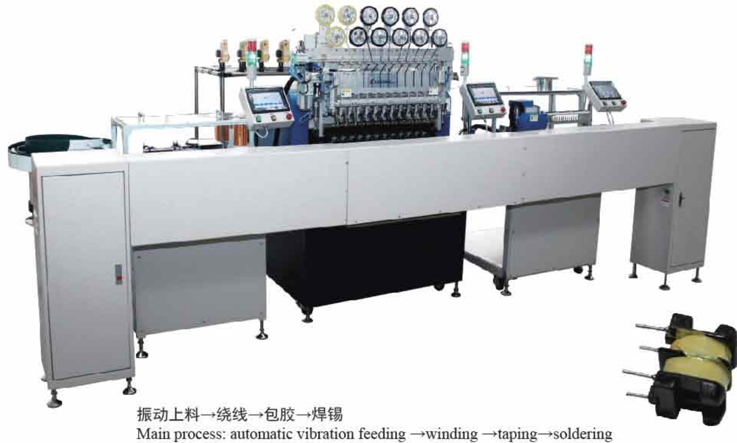
ER5012全自动滤波器流水线 ER5012 Full Automatic Production Line For Wave Filter
