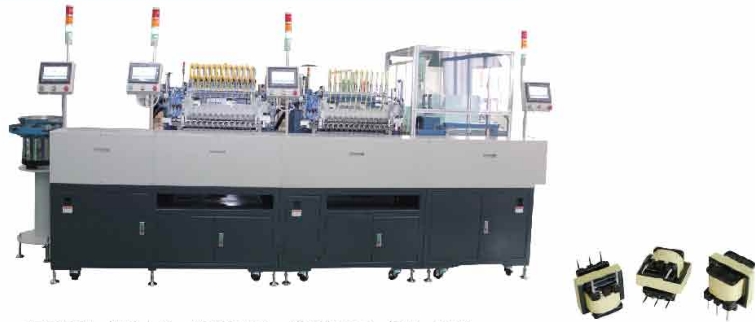
ER3712全自动EE电子变压器流水线 ER3712 Full Automatic Production Line For EE Type Transformer
