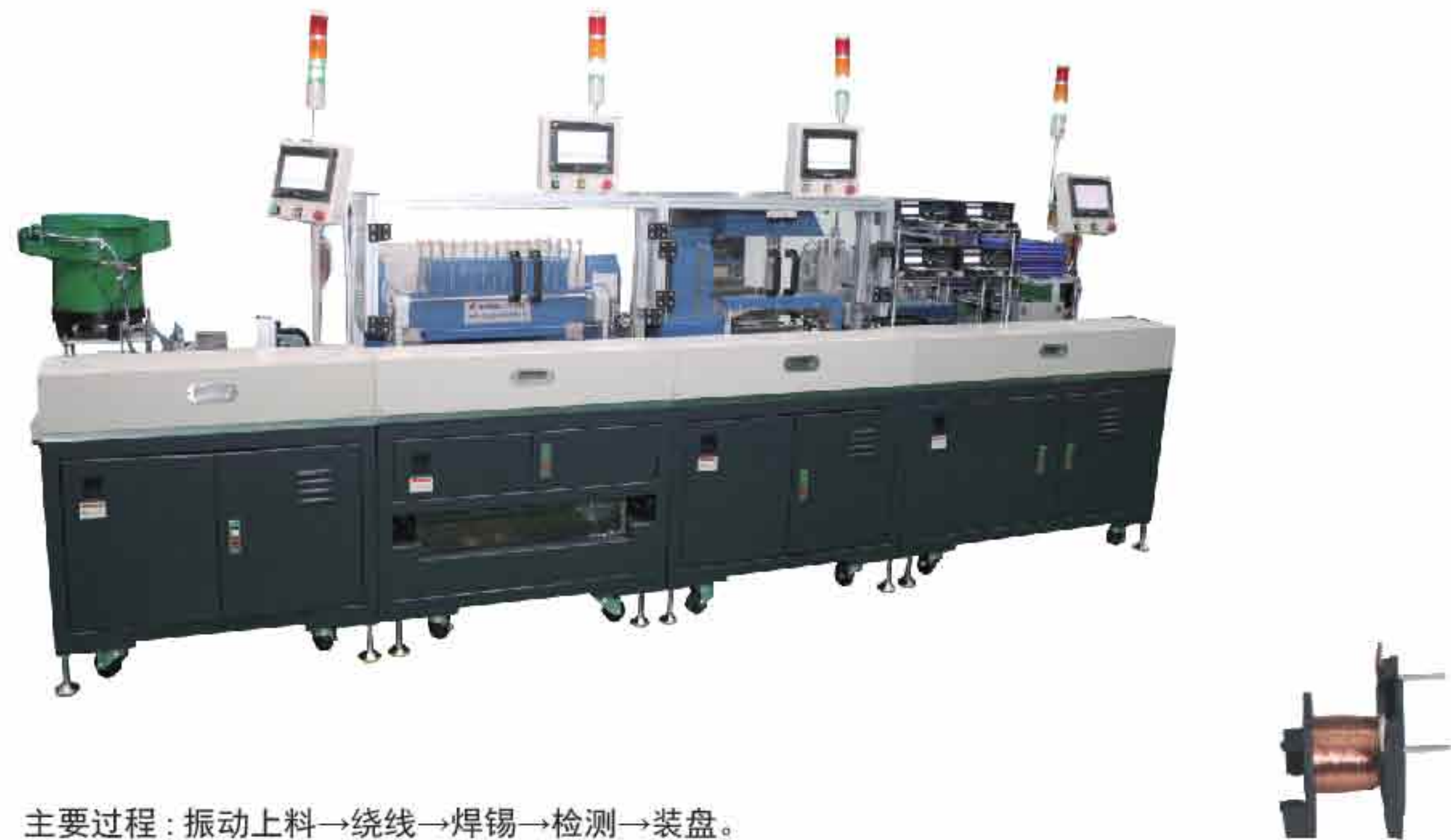
ER3016全自动继电器线圈流水线 ER3016 Full Automatic Production Line For Relay Coil
